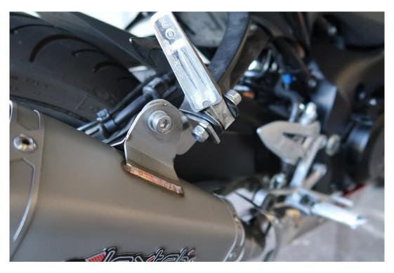
Attached the link pipe (if supplied) to the downpipe using a small amount of exhaust paste (if required), then slide the silencer over the link pipe and align with the mounting bracket as previously installed.
