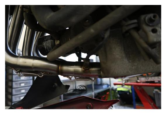
Check to clearances and tighten each of the exhausts nuts on the cylinder head to 20Nm. Add all the springs to the system to pull it tight.
