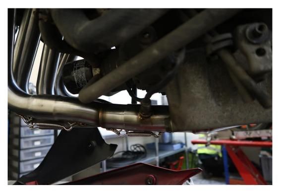
Tighten the bolt that secures the system to the frame to 20Nm as per the image below.
