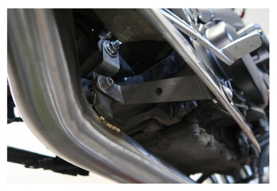
Re-install the Lambda sensor ensuring that it is done to 30Nm. See image below.
