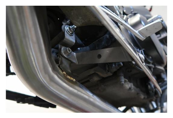
Remove the pin holding the pillion peg and replace with the M8 bolt & nut (supplied) whilst ensuring the silencer mounting bracket is attached as per the image below. Tighten the nut to a torque of 25Nm.
