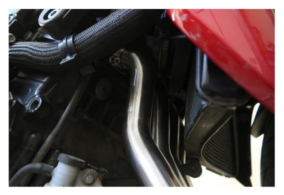
Insert 1&2 and 3&4 into the corresponding collectors but leave the springs at this stage.
