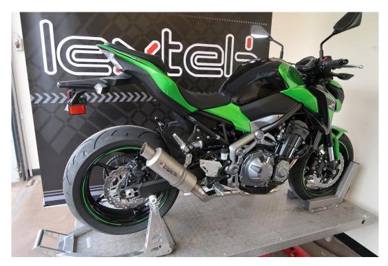
Check the clearances of the silencer against the swinging arm and other moving parts. At this stage it is easy to adjust the system to obtain clearances.
