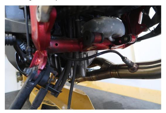
Tighten the header ports to 20Nm per nut.
