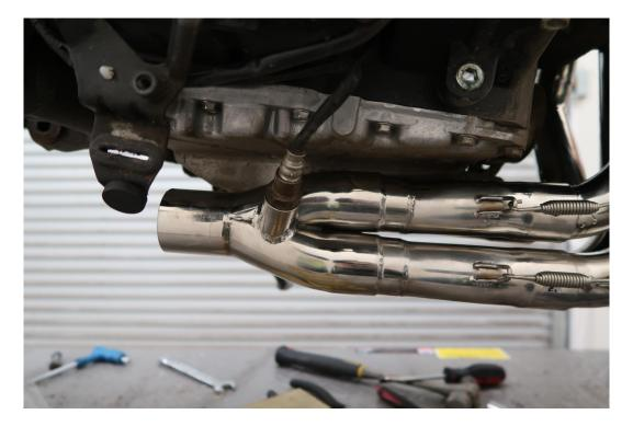
Re-install the lambda sensor and tighten to 39Nm.
