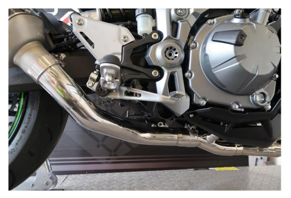
Mount your new Lextek Silencer to the header and line with the mounting point on the pillion peg. Using the OEM bolts secure the silencer.
