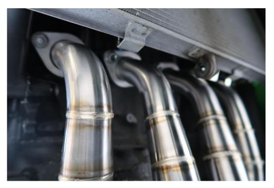
Place each header pipe into the exhaust ports and tighten the exhaust nuts. Please ensure at this point of the process they are only finger tight.
