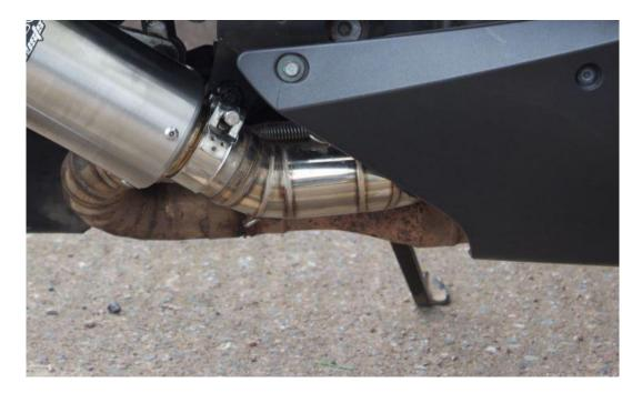
Once you are happy with the clearances then tighten both clamps to 14Nm and tighten the mounting bolt to 20Nm.
