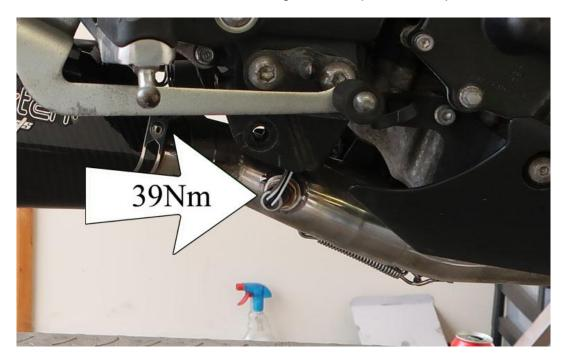
Install L-Shaped bracket onto OE mounting bracket using original bolts.
