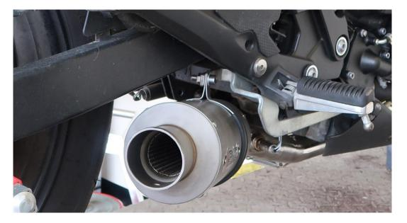
Adjust the silencer to the correct position and tighten the clamp ensuring the correct torque settings are used.
