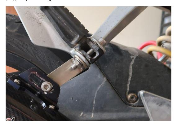
Tigthen the nut to 15Nm and check the pillion peg still functions correctly (If fitted).
