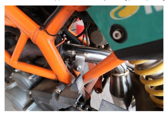
Using the OEM bolt secure the link pipe to the frame and tighten the clamp to 20Nm.
