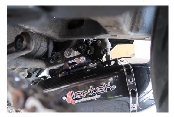
Loosely secure your new Lextek Silencer to the header using the mounting point (installed earlier).
