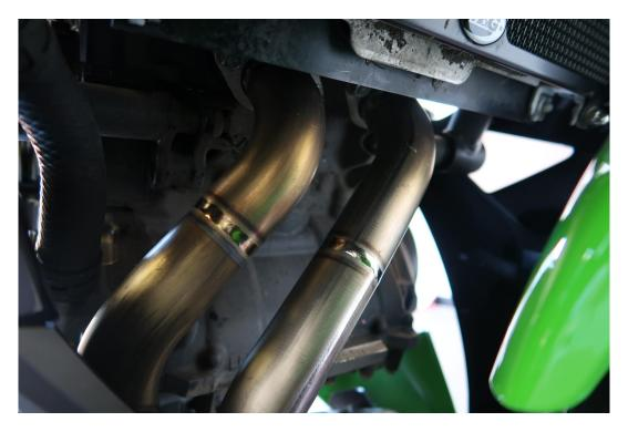
Add the middle section to the down pipes and secure with the springs provided.
