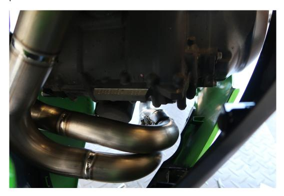
Tighten the header nuts to 20Nm torque setting and all clamps to 12Nm torque.
