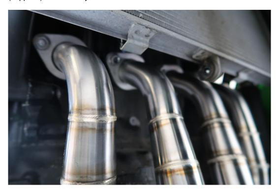
Place each header pipe into the exhaust ports and tighten the exhaust nuts. Please ensure at this point of the process they are only finger tight.
