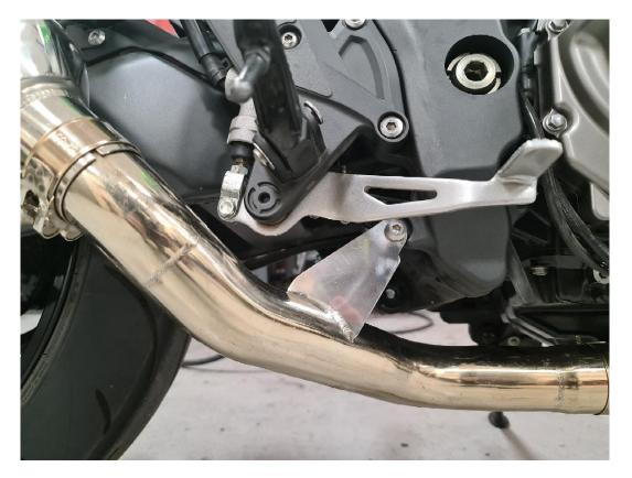
Mount your new Lextek Silencer to the header and line with the mounting point on the pillion peg. Using the OEM bolts secure the silencer, use a spacer (supplied) if needed.
