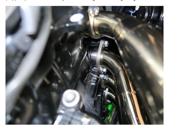
Place each header pipe into the exhaust ports and tighten the exhaust nuts. Please ensure at this point of the process they are only finger tight.
