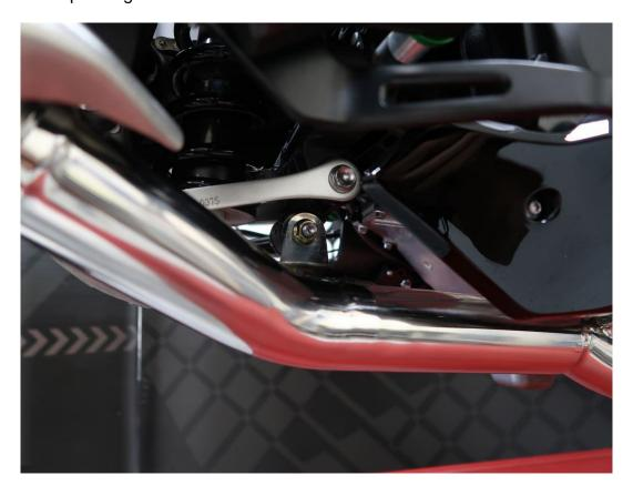
Using the OE mounting bolt and M10x1.25 nut (supplied) locate the mounting bracket and secure to frame mounting point. At this time only secure lightly to allow for adjustment
