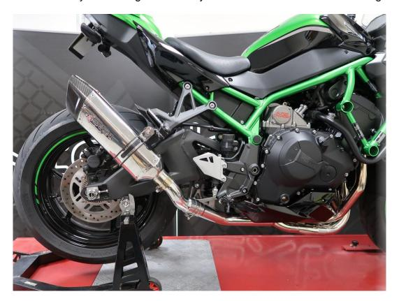
Torque the headers into the exhaust ports to 22Nm for each nut.
