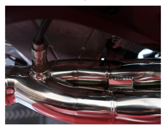
Mount your new Lextek Silencer and link pipe OR your OE silencer to the mid pipe using a small amount of paste (supplied) and align with the silencer mounting point.
