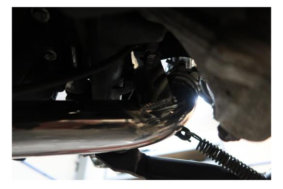
Using paste applied to the inside of the mid pipe and the supplied connection clamp, assemble the link pipe to mid pipe connection. And mount the silencer using paste and clamp as supplied.
