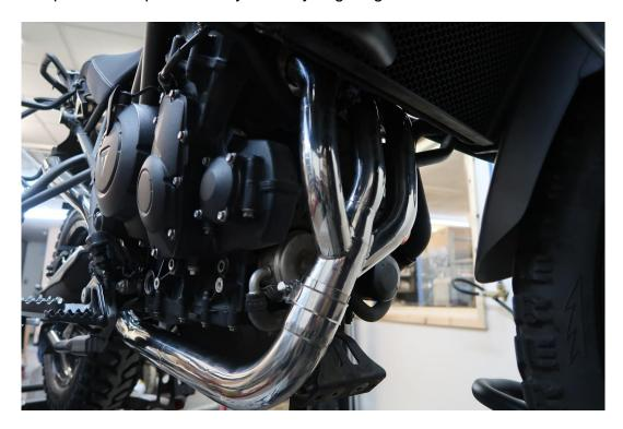
Using paste applied to the inside of the mid pipe connection and supplied connection clamp assemble the mid pipe to header connection and hang the mid pipe on its rear mounting point. Retain with the mounting fixings but do not tighten fully at this stage
