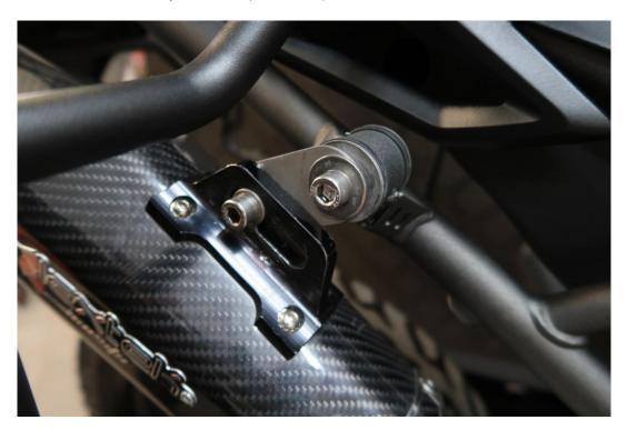
Finally, starting at the silencer, ensure all pipework is oriented to allow clearances to other parts of the bike along its routing and secure all fixings, mounting bolts, clamps and header nuts are tightened.
