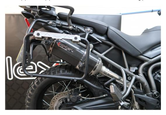
\*Note\* If using a silencer requiring additional mounting brackets ensure the silencer is connected to the outside of any bracket (as below)
