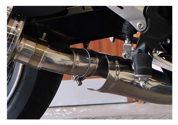
Slide the inlet of the silencer onto the link pipe until it stops, then adjust the silencer AND link pipe to ensure clearance to the swinging arm and its proximity to the silencer mounting on the pillion peg. Using the fixings (supplied) to mount the silencer to the bike as per the photos below.
