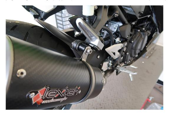
Now the silencer is in the correct position all the fixings need to be secured. i.e.  $2 \times 10^{-2}$  x clamps and exhaust strap.
