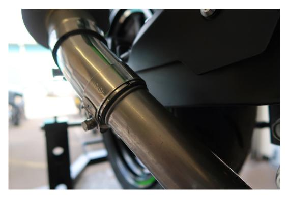
Slide the inlet of the silencer onto the link pipe until it stops, then adjust the silencer AND link pipe to ensure clearance to the swinging arm and its proximity to the silencer mounting on the pillion peg. Using the fixings (supplied) to mount the silencer to the bike as per the photo below.
