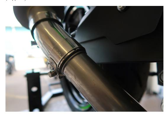
Slide the inlet of the silencer onto the link pipe until it stops, then adjust the silencer AND link pipe to ensure clearance to the swinging arm and its proximity to the silencer mounting on the pillion peg. Using the fixings (supplied) to mount the silencer to the bike as per the photo below.
