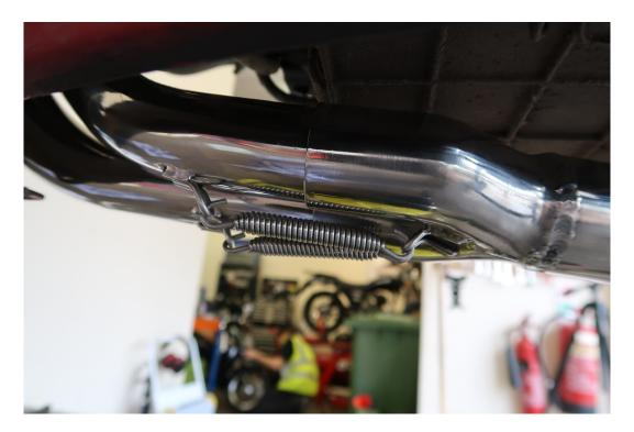
Check the exhaust system for clearances between the exhaust and frame, engine and fittings. Adjust if necessary.
