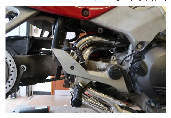
Insert the exhaust gaskets (supplied) into the front exhaust ports, use a small amount of exhaust paste to hold them into the ports if required.
