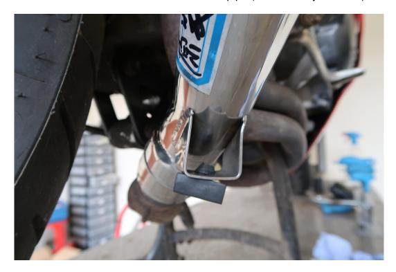
Slide the clamp onto the link pipe and slide over the outlet from the down pipe.
